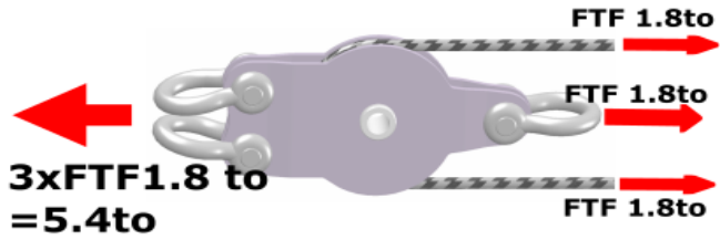
Figure 1: Forces acting on a single sheave pulley
